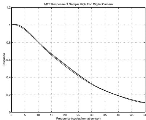
Figure 4. Sample RGB MTF output from an ESC.
