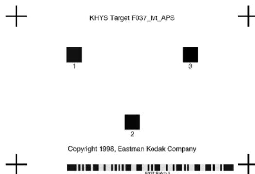
Figure 8. Sample veiling flare target with three different density patches.
