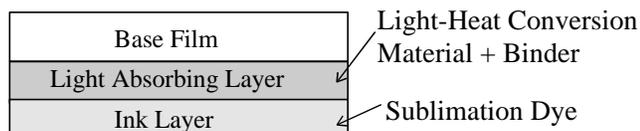
Figure 2. A double layered ink donor sheet for laser dye thermal transfer printing.
