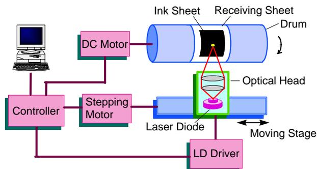
Figure 3. A schematic diagram of the laser thermal dye transfer printing system.
