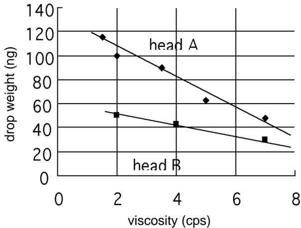
Figure 3. The relationship between viscosity and droplet size
