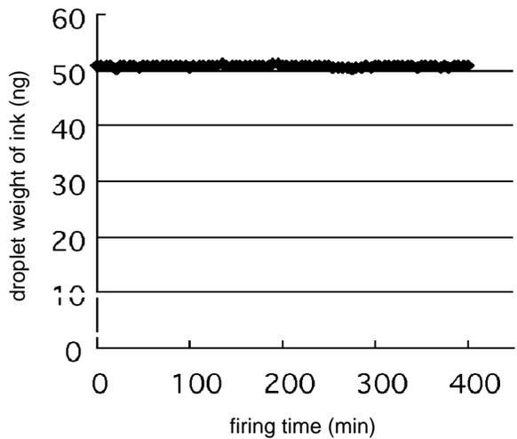
Figure 8. The weight change of droplet during firing
