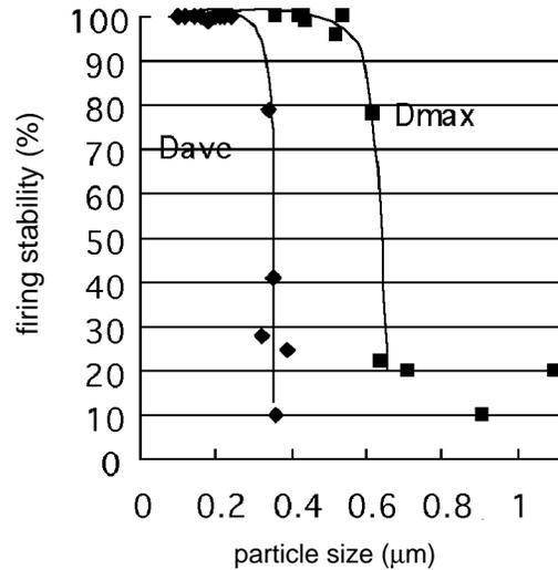
Figure 4. Dependence of firing upon particle size of dispersed dye
