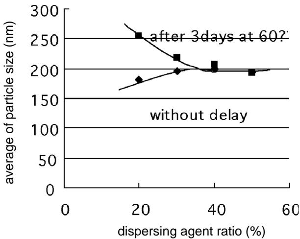
Figure 6. Dependence of aggregation upon the ratio of dispersing agent at accelerate condition
