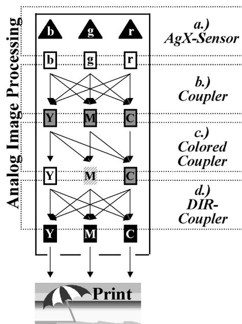
Figure 1. Analog image processing in a conventional color negative film during the photographic processing (symbols are explained in Figure 2).
