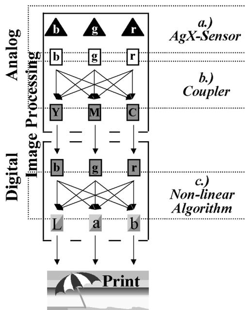
Figure 3. Separation of image processing of a scan film in an analog and a digital part.
