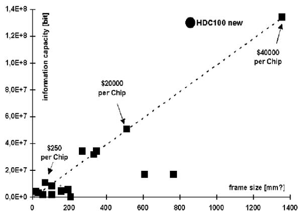
Figure 4. Comparison of information capacity vs. frame size of digital sensors (CCD and CMOS, rectangular dots) with a conventional silverhalide negative film (circular dot).
