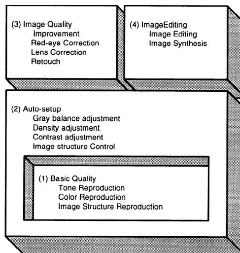
Figure 2. Frontier 350 image processing
