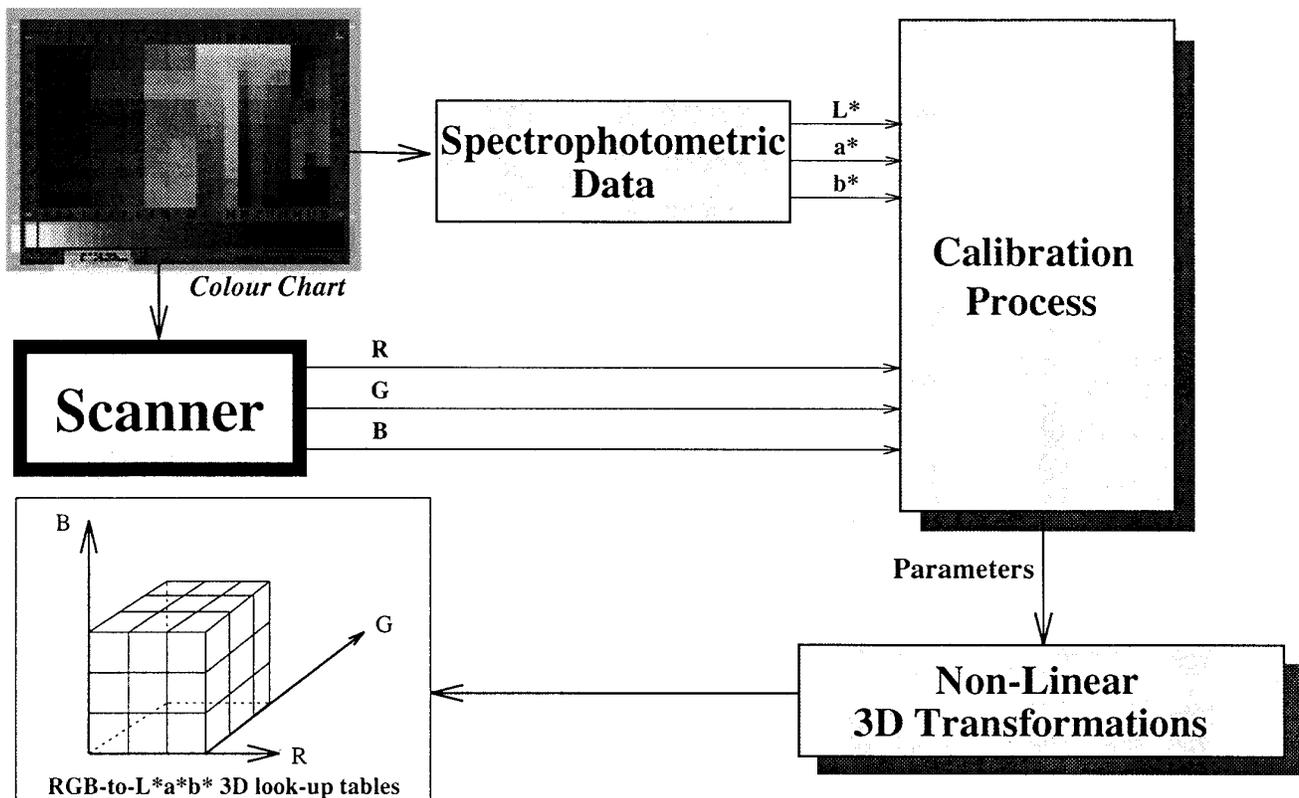
Figure 2. The scanner calibration process, providing a 3D look-up table for the conversion from scanner RGB to CIELAB.
