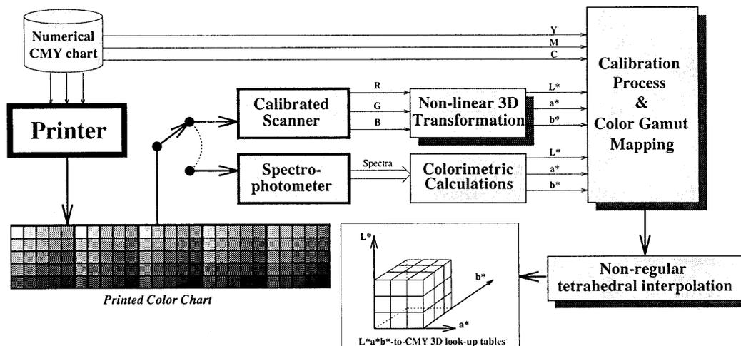
Figure 4. The printer calibration process, providing a 3D lookup-table for the conversion from CIELAB to CMY.
