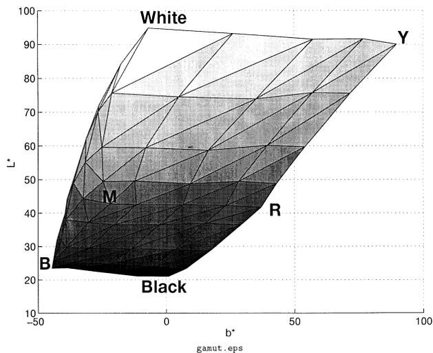
Figure 5. A CIELAB view of the triangulated color gamut of the Mitsubishi S340-10 sublimation printer, built on a regular  $5 \times 5 \times 5$  color chart.
