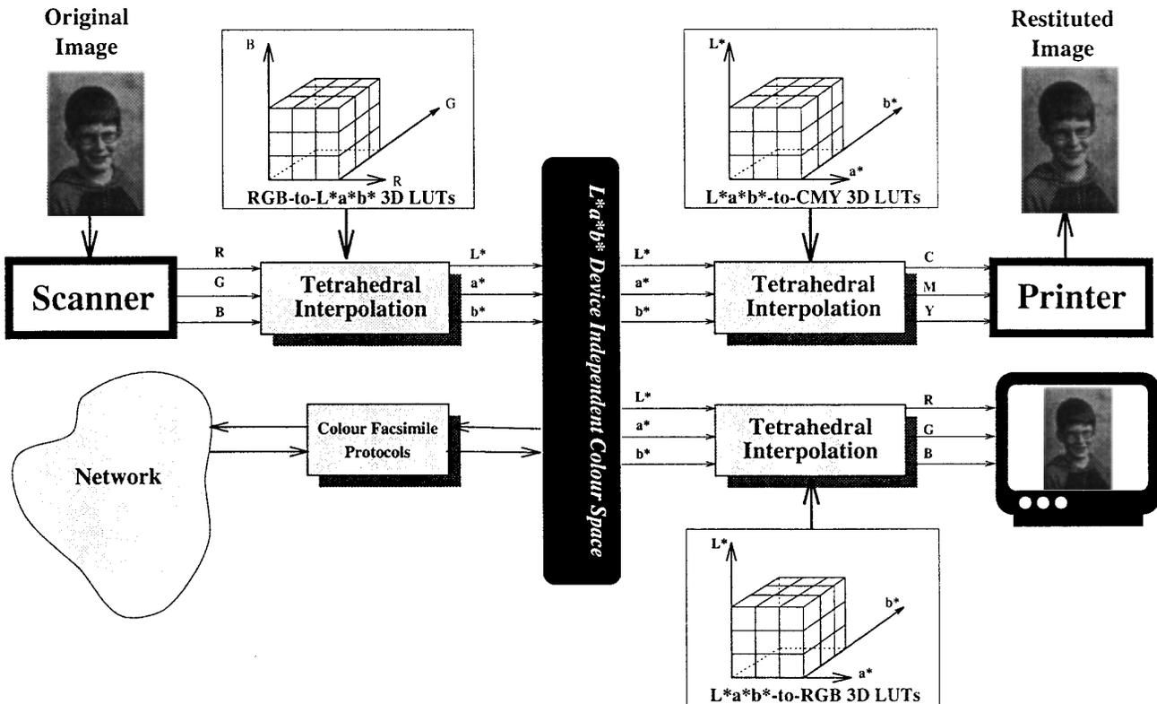
Figure 1. A color facsimile system. The transformations between device dependent color coordinates (RGB and CMY) and the CIELAB color space is performed using 3D look-up tables and a tetrahedral interpolation technique.
