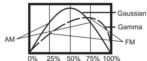
Figure 2. Dot-gain for a colorant consisting of 25% of one primary colorant and 75% of another
