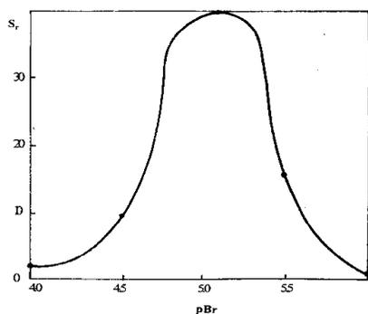
Figure 4: variation of speed with PBr, the amount of sulfur sensitizer added was  $4.0 \times 10^{-3}$  mol  $\text{Na}_2\text{S}_2\text{O}_3$ /mol AgBr and sensitization period was 30 minute at  $55^\circ\text{C}$ .
