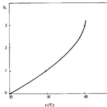
Figure 2: variation of speed with ripening temperature, the amount of sulfur sensitizer added was  $4.0 \times 10^{-3}$  mol  $\text{Na}_2\text{S}_2\text{O}_3$ /mol AgBr and sensitization period was 30 minute.
