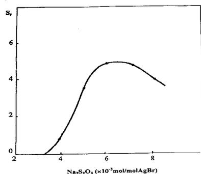
Figure 1: variation of speed with  $\text{Na}_2\text{S}_2\text{O}_3$  amount, the sensitization period was 30 minute at 55°C.
