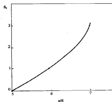
Figure 3: variation of speed with PH, the amount of sulfur sensitizer added was  $4.0 \times 10^{-3}$  mol  $\text{Na}_2\text{S}_2\text{O}_3$ /mol AgBr and sensitization period was 30 minute at 55°C.
