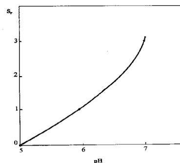
Figure 3: variation of speed with PH, the amount of sulfur sensitizer added was  $4.0 \times 10^{-3} \text{ mol Na}_2\text{S}_2\text{O}_3/\text{mol AgBr}$  and sensitization period was 30 minute at 55°C.
