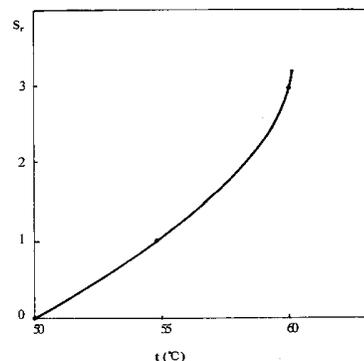
Figure 2: variation of speed with ripening temperature, the amount of sulfur sensitizer added was  $4.0 \times 10^{-3} \text{ mol Na}_2\text{S}_2\text{O}_3/\text{mol AgBr}$  and sensitization period was 30 minute.
