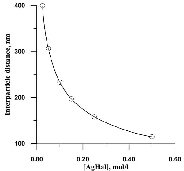
Figure 2. The calculated dependence of interparticle distance in gel on concentration of a silver halide (microcrystals average size is 50 nm).
