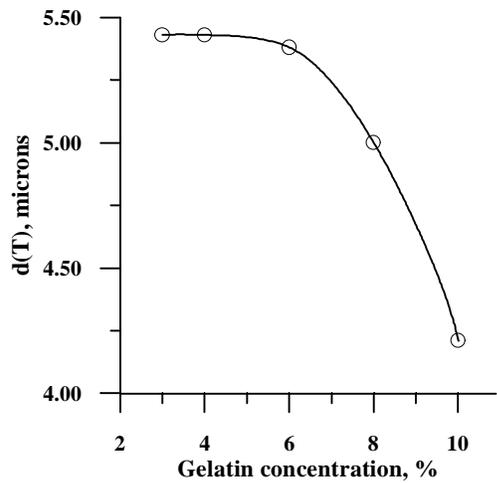
Figure 6. The dependence of an average equivalent diameter of tabular crystals on concentration of a gelatin. The initial fine emulsion characteristics: microcrystal size - 52 nm, 76,000 microcrystal per nucleus, microcrystal concentration -  $1.11 \cdot 10^{17} l^{-1}$ .
