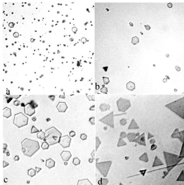
Figure 4. The microphotos (x1000) of crystal received by recrystallization in gel (pBr=1.0; gelatin concentration 3 %) and by physical ripening (d). The microcrystal concentration:
