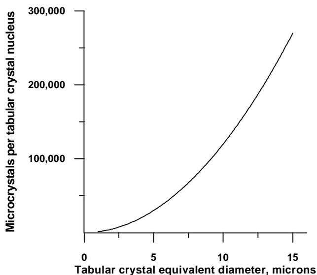
Figure 3. The calculated dependence of amount of microcrystals of a fine emulsion per one tabular crystal on an average equivalent diameter of this tabular crystal (microcrystal size is 50 nm, tabular crystal thickness is 100 nm).
