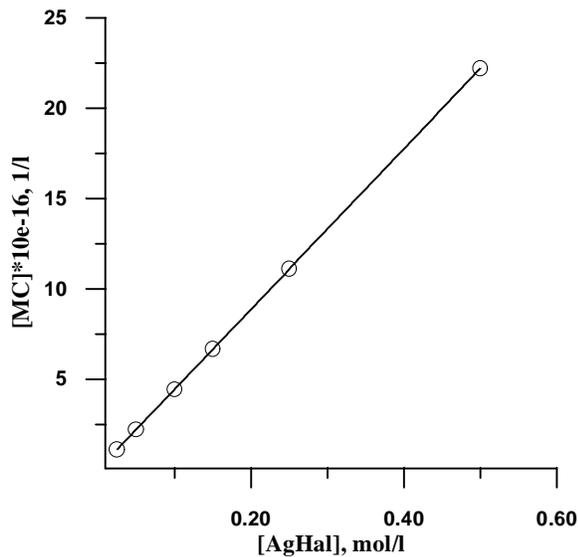
Figure 1. The calculated dependence of microcrystal concentration in gel on silver halide concentration (microcrystal size is 50 nm).
