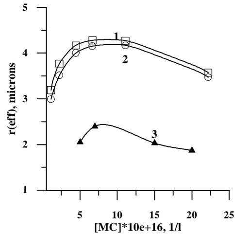
Figure 7. The dependence of effective radius of action of a tabular crystal nucleus on microcrystal concentration. The initial emulsion characteristics: 1 - 76,000 microcrystal per nucleus, microcrystal size 52 nm; 2 - 73,000 microcrystal per nucleus, microcrystal size 50 nm; 3 - reference 1.
