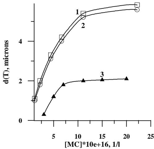
Figure 5. The dependencies of an average equivalent diameter of tabular crystals on concentration of microcrystals in gel. The initial emulsions characteristics: 1 - 76,000 microcrystal per nucleus, microcrystal size 52 nm; 2 - 73,000 microcrystal per nucleus, microcrystal size 50 nm; 3 - reference 1.
