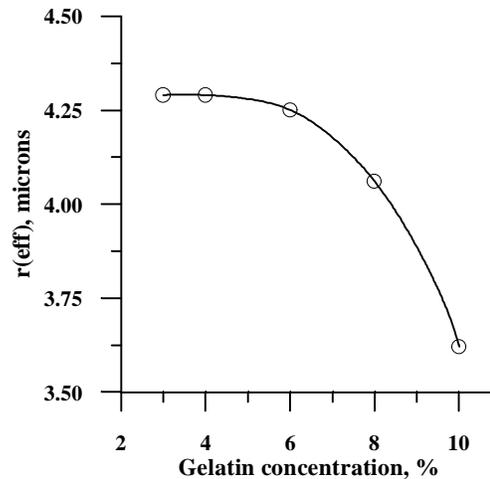
Figure 8. The dependence of effective radius of action of a tabular crystal nucleus on gelatin concentration. The initial emulsion characteristics: microcrystal size is 52 nm, 76,000 microcrystal per nucleus, microcrystal concentration is  $1.11 \cdot 10^{17} l^{-1}$ .
