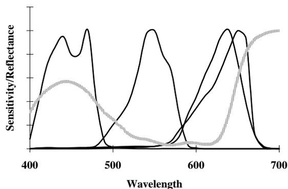
Figure 6. A multilayer film spectral sensitivity showing the shortened red response achieved with the mixed aggregate of dyes 1 and 2 in Figure 4. The broad jagged line is the reflectance spectrum of the lobelia flower
