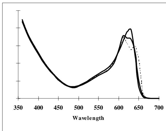
Figure 5. The effect of dye addition order for dyes 1 and 2 on the resulting absorption spectrum of the dyed, coated emulsion. Curve A (solid) - Dye 1 added first, then dye 2 after 15 min. Curve B (dashed) - Dye 2 added first, then dye 1 added after 15 min. Curve C (bold) - Both dyes added simultaneously and held 30 min.
