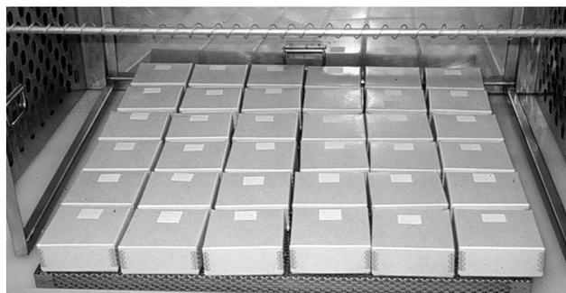
Figure 5. Arrangement of boxed samples in incubation chamber. Spacing boxes a half-inch apart on raised rack permitted free flow of air around samples.
