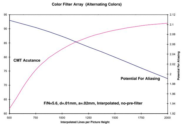
Figure 19. The CMT Acutance and Potential for Aliasing for a DSC with a Color Filter Array.
