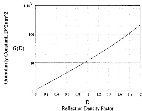
Figure 5: G-D at graininess threshold. Below curve GS is not visible.
