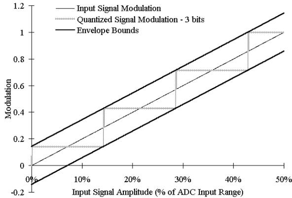
Figure 5. The calculated envelope versus input signal amplitude for a 3 bit quantization stage. The mean level of the input signal is kept constant at 50% of the input range of the ADC.
