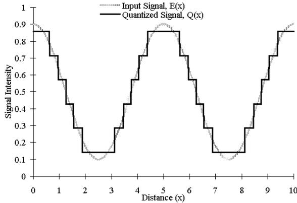
Figure 1. A sinusoidal input signal of modulation 0.8 ( $a=0.5$ ,  $b=0.4$ ) and its corresponding output when quantized using 3 bits. The input range of the quantizer is normalized so that  $I_{MAX}=1$ .
