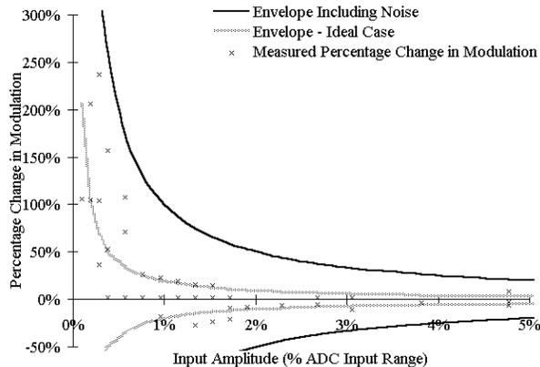
Figure 8. Percentage change in the input signal modulation versus input signal amplitude for the 8 bit ADC. The theoretical bounds calculated for an ideal and noisy system are also shown.
