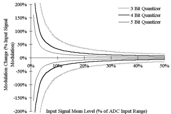
Figure 6. The calculated envelope versus input signal amplitude for 3, 4 and 5 bit ADCs.
