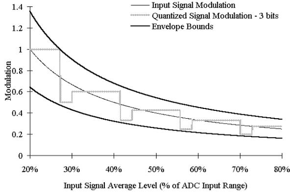
Figure 4. The calculated envelope versus mean input signal level for a 3 bit ADC. Input signal amplitude is kept constant at 20% of the input range of the ADC.
