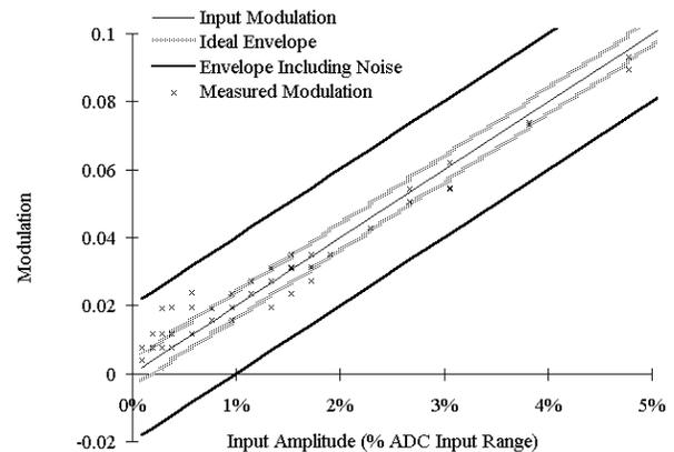
Figure 7. Measured quantized signal modulation versus input signal amplitude for the Ferantti ZN449E 8 bit ADC. Also shown are the theoretical bounds calculated for an ideal and noisy system.
