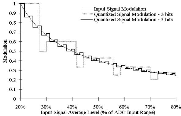
Figure 2. Input signal modulation and quantized signal modulation versus mean input signal level. The amplitude of the input signal is constant at 20% of the input range of the ADC.
