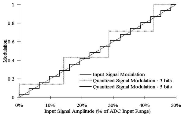
Figure 3. Input signal modulation and quantized signal modulation versus input signal amplitude. The mean level of the input signal is kept constant at 50% of the input range of the ADC.
