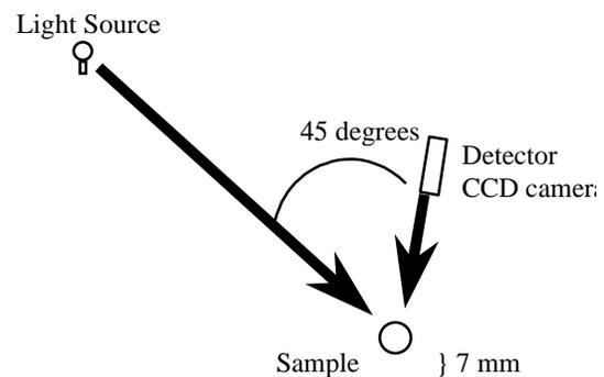
Figure 2. Configuration for the micro-goniophotometer.
