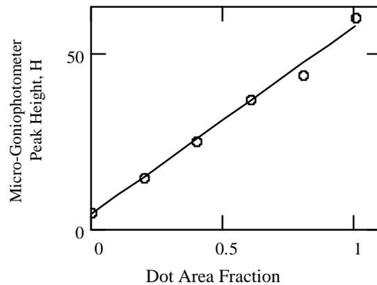
Figure 6. Gloss as a function of dot area fraction for a halftone image made by a phase change ink jet system.
