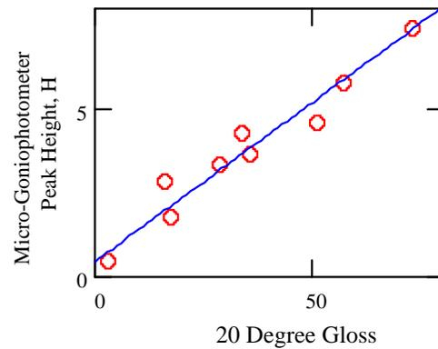
Figure 5. Correlation between the height of the gloss peak and independently measured values for 20 degree gloss.
