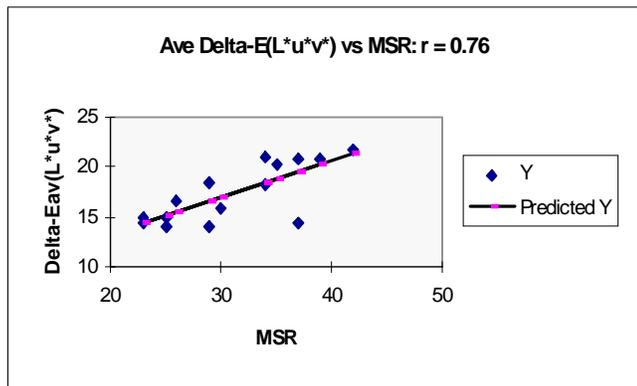
Fig 2 : Scatter-plot of  $\Delta E_{av}(L^*u^*v^*)$  vs. MSR
