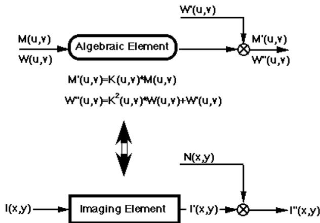
Figure 2. Linear stationary model of Imaging element as implemented in IQA Process Control .
