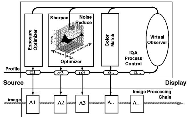
Figure 1. IQA architecture: A<sub>i</sub> represent Image processing filters in the image processing chain;  $\alpha_i$  represent algebraic models of the Image processing filters in the image processing chain.
