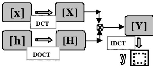
Figure 2: Linear filtering or convolution in the DCT domain.
