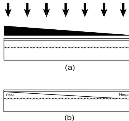
*Fig.1; Geometrical noise in photographic film images. A wedge exposure to a film with coating non-uniformity (a) results in a posi image with geometrical noise which becomes relatively larger toward highlight (b).*
