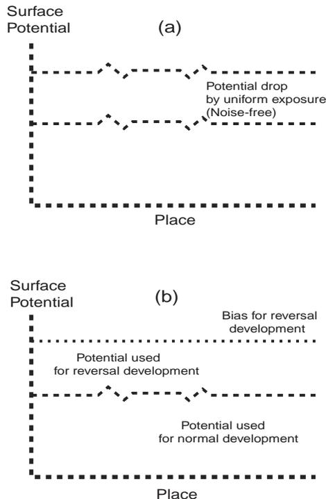
Fig.2; Surface potential of a xerographic photo-sensor before and after a uniform exposure (a), and the potential used for normal or reversal development.
