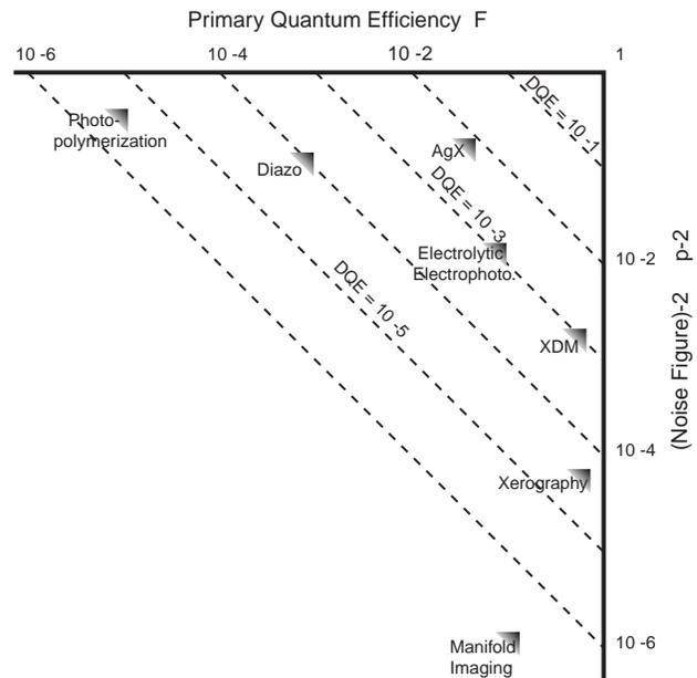
Fig.3; Characterization of various imaging systems in terms of primary quantum efficiency and internal noise.
