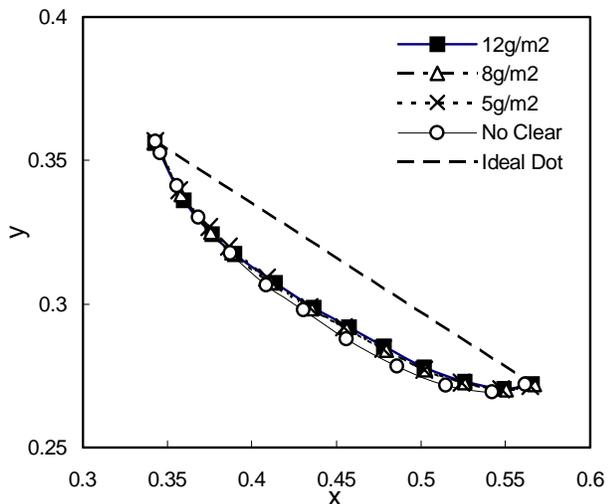
Figure 3: CIE x-y chromaticity coordinates of halftone magenta step wedges on which the clear toner was developed as a parameter of the mass density of clear toner.
