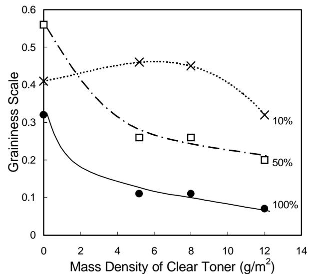
Figure 2 : The graininess of the halftone images as a function of the mass density of clear toner. The number in this figure means the magenta image coverage.
