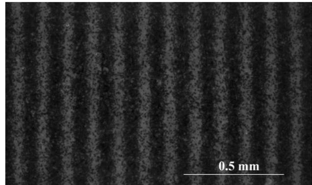
Figure 4: The Microphotograph of the 50% coverage Magenta image with the clear toner of 12.0g/m<sup>2</sup> developed mass
