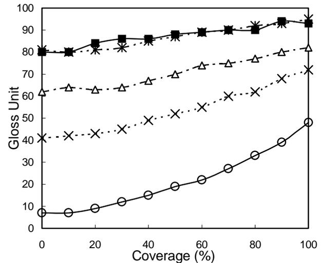
Figure 1: The gloss of magenta step wedges on which the clear toner developed in several different mass density as a function of magenta image coverage. Parameters are as follows ;
