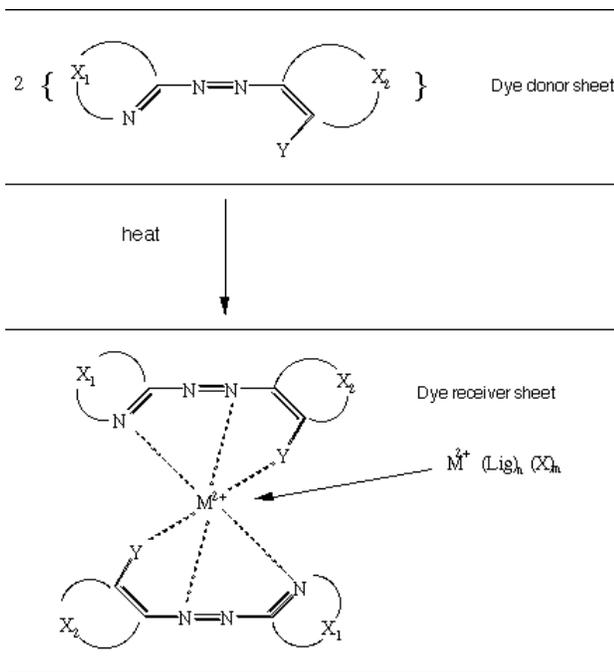
Fig. 4 Principle of post-chelate process
