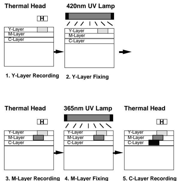
Figure 2: Image-forming process by the TA system
