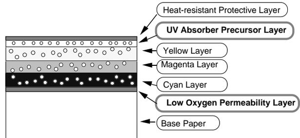
Figure 9: Simplified cross-sectional view a new type of TA paper
