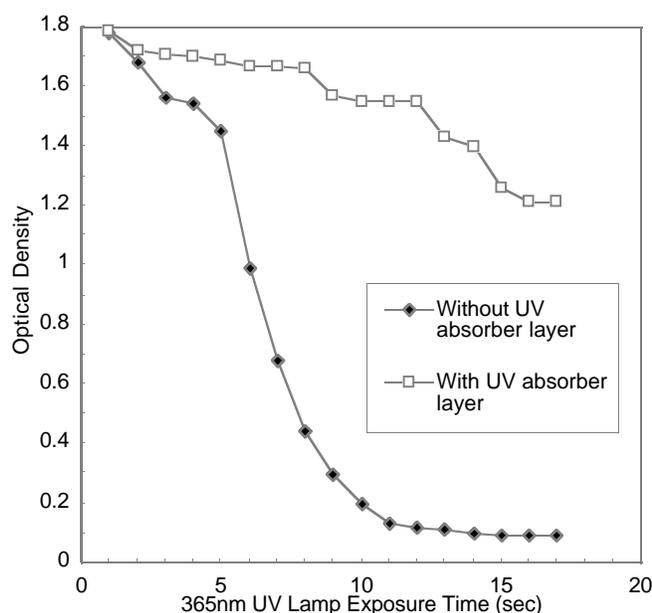
Figure 3: Effect of the ultraviolet absorber layer for the magenta color forming layer fixation.
