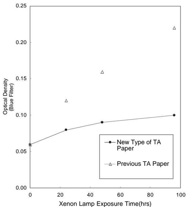
Figure 8: Background coloration of a new type of TA paper
