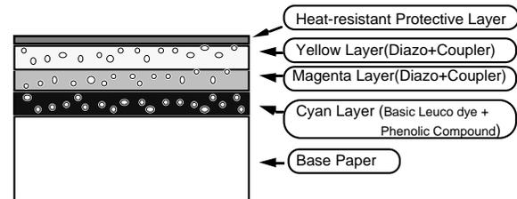
Figure 1: Simplified cross-sectional view of TA paper
