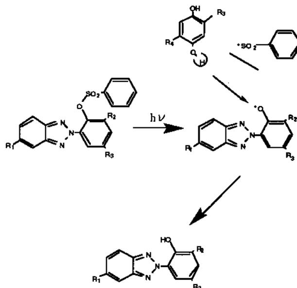
Figure 4: The typical ultraviolet absorber precursor and its conversion scheme to the ultraviolet absorber
