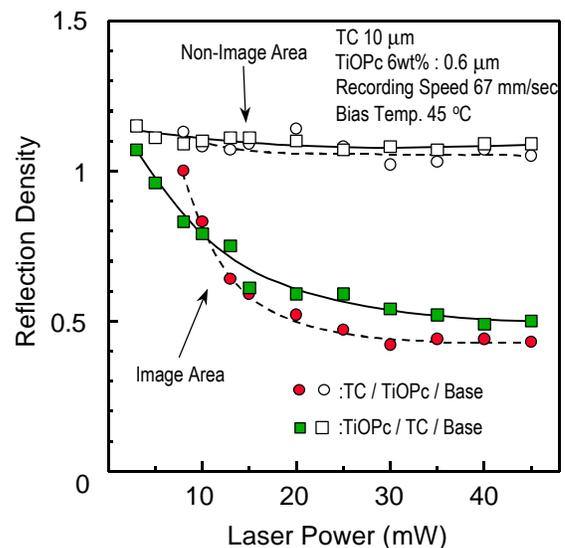
Figure 5. Relationship between reflection density and laser power for the double-layered thermo-rewritable sheet.
