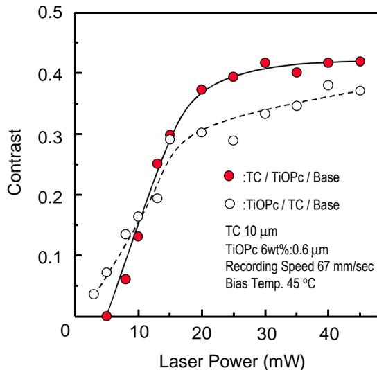
Figure 6. Relationship between an optical reflection contrast and laser power for the double-layered thermo-rewritable sheet.
