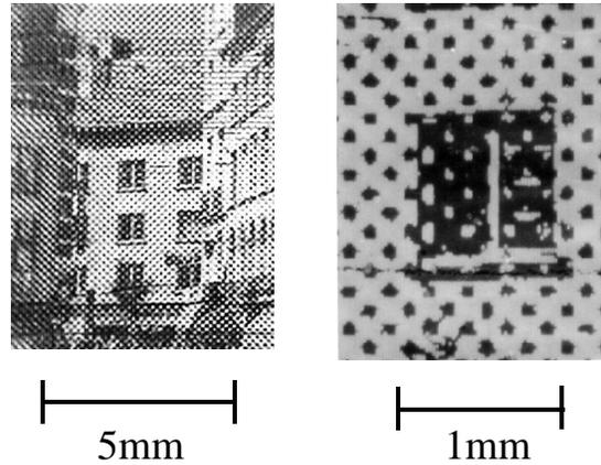
Figure 7. Microphotographs of printed samples. Image resolution:1524dpi, Half Tone:180lines/inch, Laser Power:25mW, Recording Speed:67mm/sec, Laser pulse width:249 $\mu$ s, Bias temp.:45°C.
