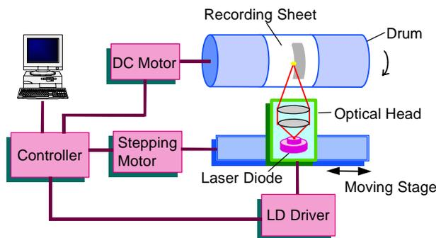
Figure 4. Schematic diagram of experimental recording system.
