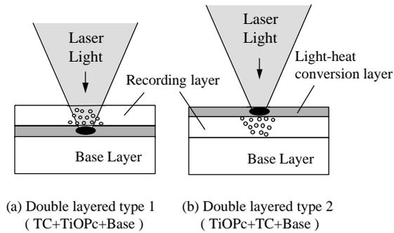
Figure 3. The construction of the double-layered thermo-rewritable sheet.
