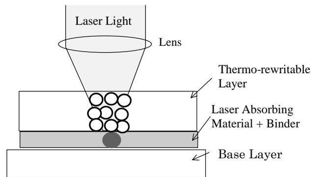
Figure 1. The principle of laser thermal Recording on Thermo-rewritable media.
