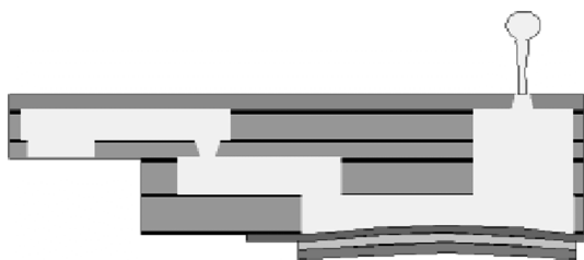
Figure 2. Cross-section of piezoelectric firing chamber
