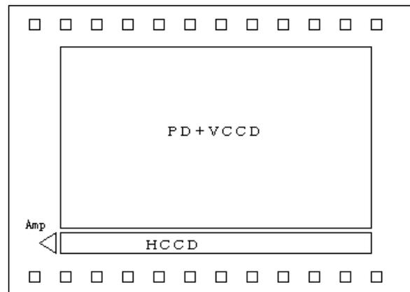
Figure 1. CCD Configuration
