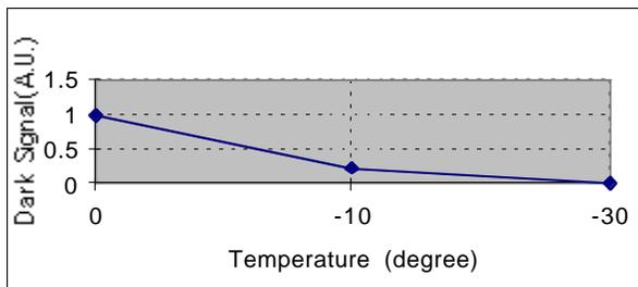
Figure 2. Dark Signal vs. Temperature
