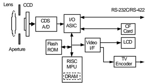
Figure 2: Image capture, processing, storage, and transmission
