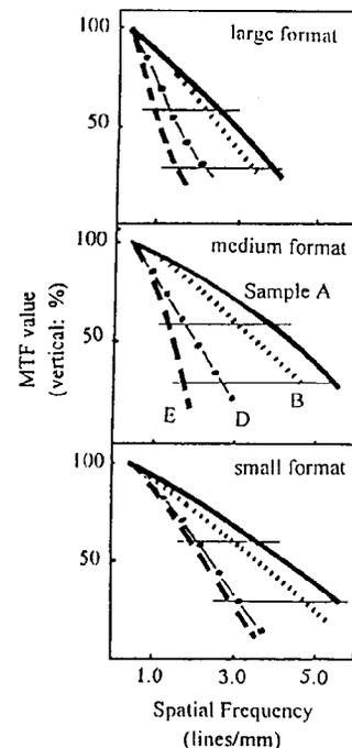
Figure 4. MTF Characteristics of sample prints.
