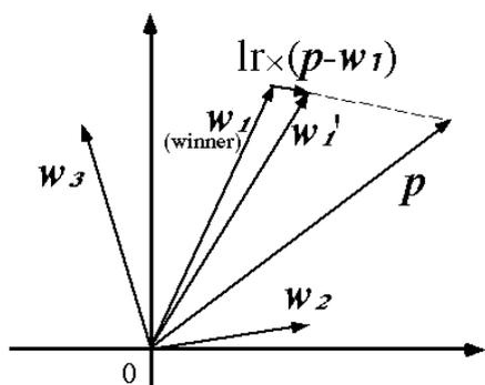
Figure 7: An example of learning step where the 2-dimensional weight vector and 3 neurons with  $\min(\|p - w_i\|) = \|p - w_1\|$  are considered.
