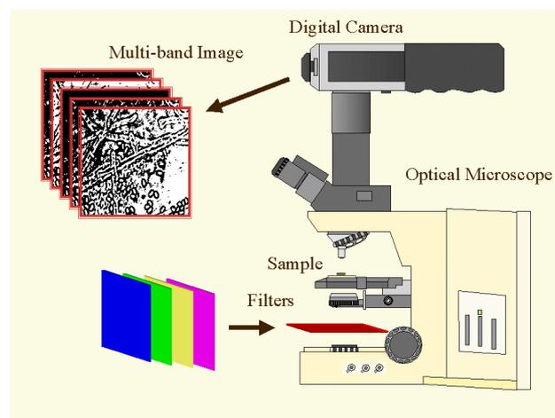
Figure 1: Imaging system to take multi-band image.
