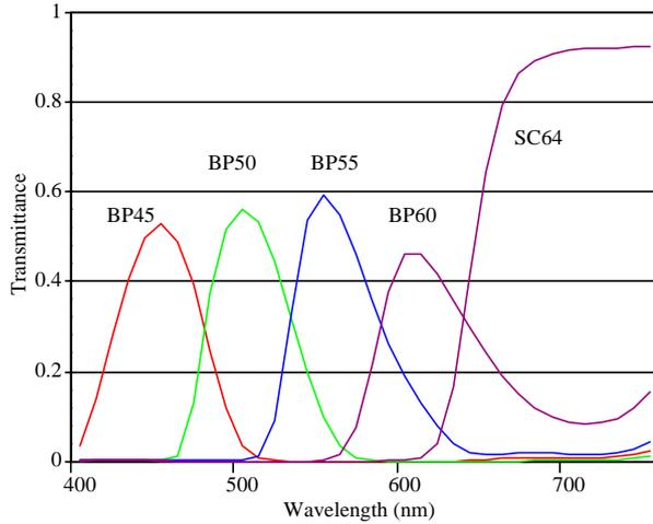
Figure 2: Spectral transmittance of five filters.
