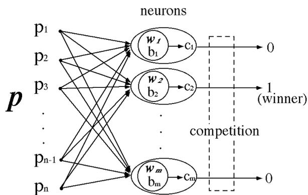
Figure 6: The architecture of the neural network used in the competitive learning method, in case of  $\max(c_i) = c_j$ .
