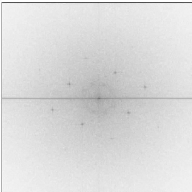
Figure 4: FFT Signature of Latent Print with High Frequency Halftone Background
