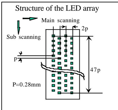
Figure 1. Layout of the LED elements
