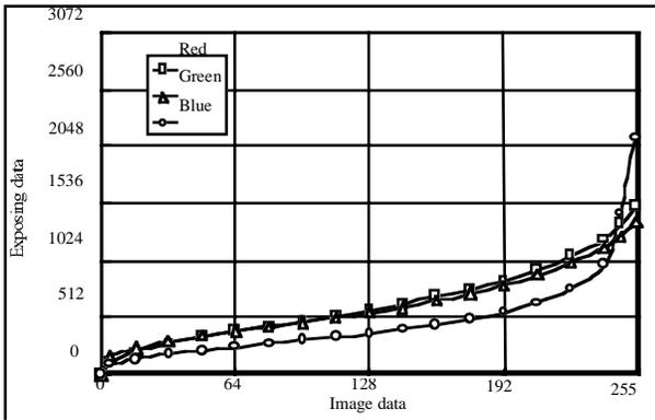
Figure 6: An example of normal 1D-LUT curve
