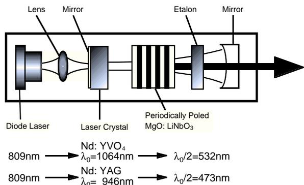
Figure 3: Schematic structure of green and blue intra-cavity SHG lasers used in the Frontier photo printer.
