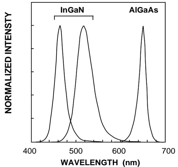
Figure 2: Emission spectra of green and blue InGaN SQW LEDs, and red AlGaAs LEDs.
