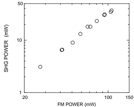
Figure 6: SHG light (475 nm) output as a function of power of fundamental light (950 nm) in waveguide SHG device fabricated on 3°-off X-cut MgO: LN.
