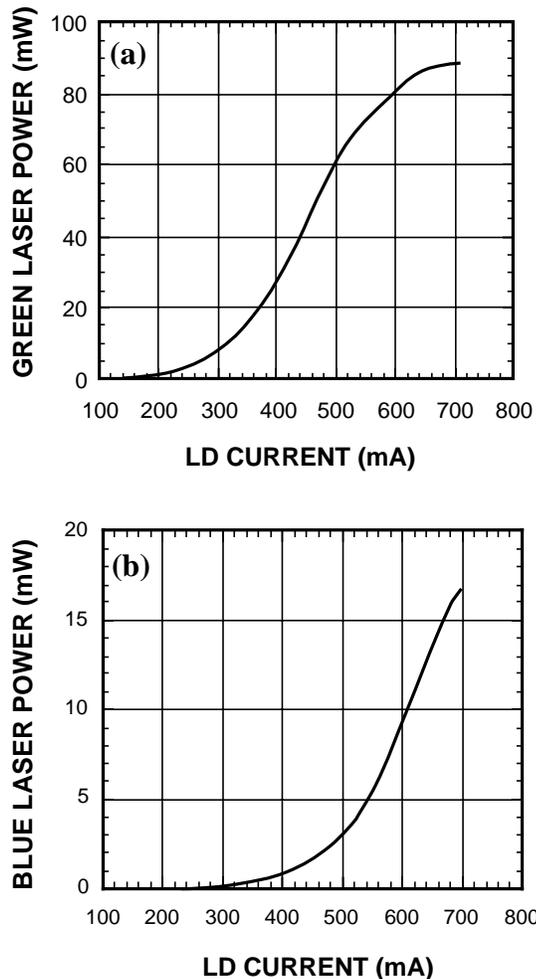
Figure 4: Light output of intra-cavity (a) green and (b) blue SHG lasers as a function of laser diode driving current.
