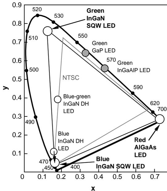
Figure 1: Chromaticity diagram in which green and blue InGaN LEDs, red AlGaAs LEDs are compared with conventional green GaP and InGaAlP LEDs and NTSC color space.
