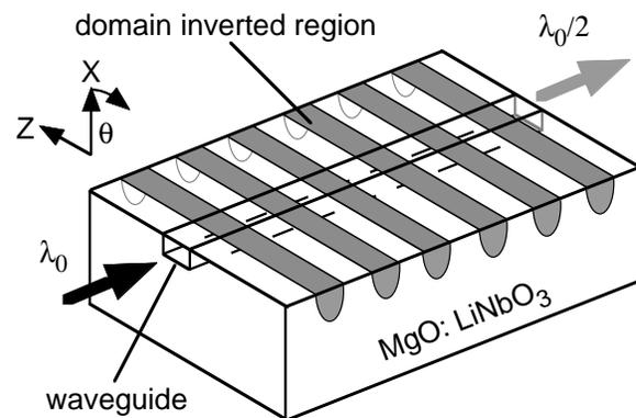
Figure 5: Schematic structure of waveguide-type SHG device using x-cut MgO: LiNbO<sub>3</sub>.
