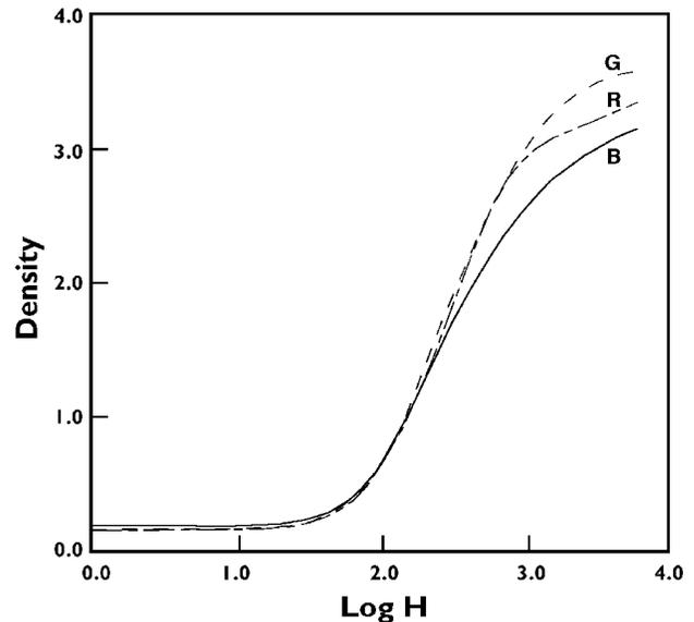
Figure 5. KODAK PROFESSIONAL Digital Paper, Type 2976 with laser sensitometer.
