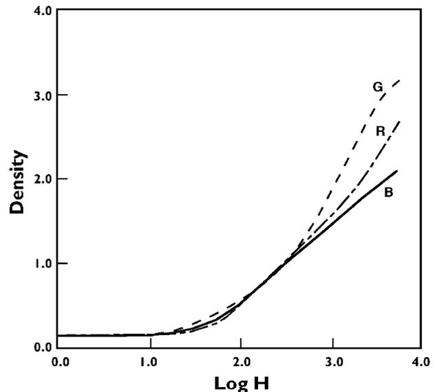
Figure 3. KODAK EKTACOLOR ULTRA II Paper with laser sensitometer.
