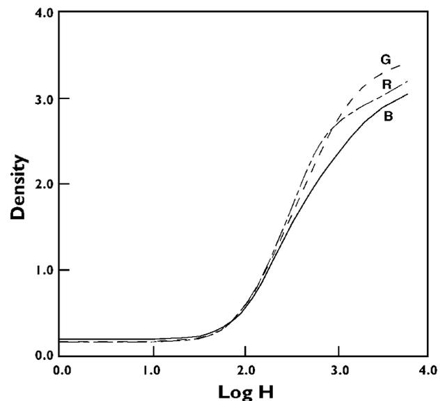
Figure 4. KODAK PROFESSIONAL Digital Paper, Type 2933 with laser sensitometer.
