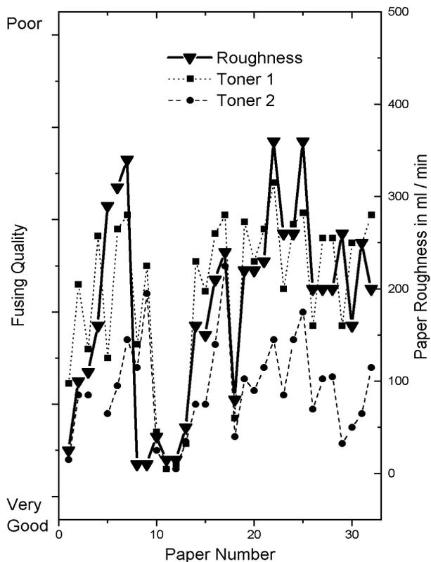
Figure 5. Integral fusing quality for 32 papers and two different toners superimposed by the paper roughness plot.
