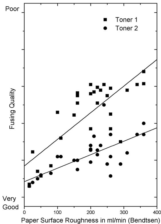
Figure 6. Integral fusing quality versus paper roughness
