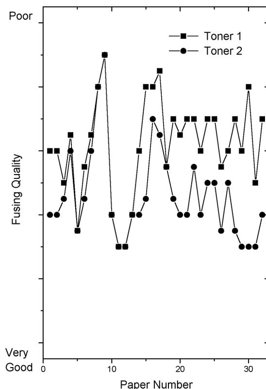
Figure 2. Fusing quality: Fold test for 32 papers and two different toners.
