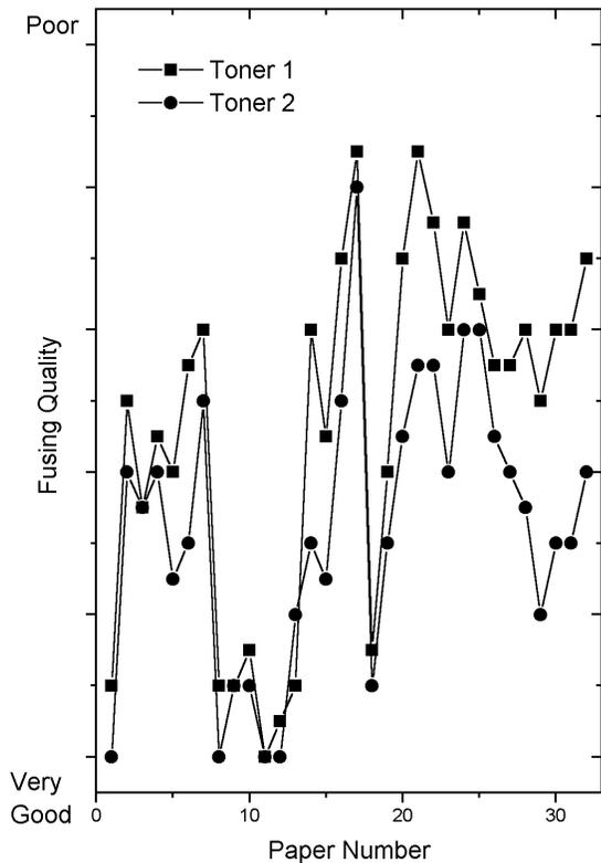
Figure 3. Fusing quality: Friction test for 32 papers and two different toners.
