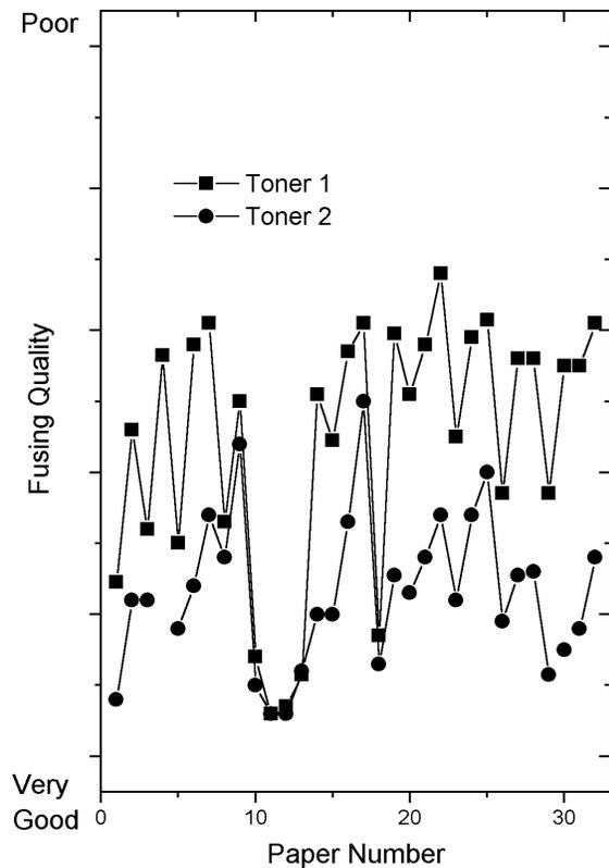
Figure 4. Integral fusing quality for 32 papers and two different toners.
