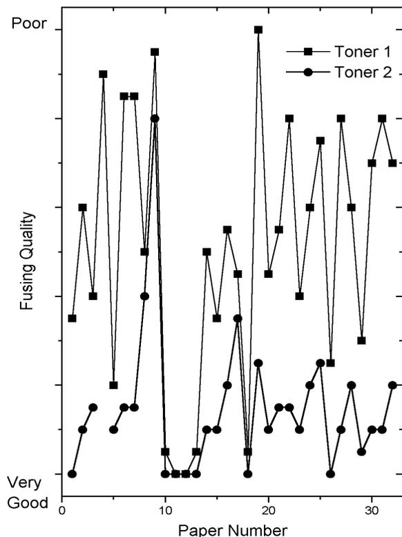
Figure 1. Fusing quality: Scotch tape test for 32 papers and two different toners.
