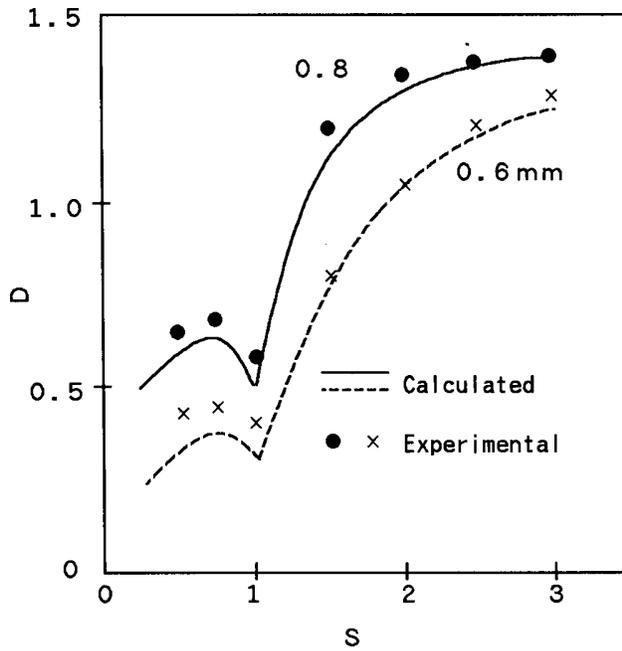
Figure 6. Influence of doctor gaps. Experimental and calculated conditions ( $V_r$ , 75 V;  $G_{dev}$ , 1 mm;  $P_1 \cdot u/\psi$ , 0.15 and 0.22 for  $G_{doc} = 0.6$  and 0.8 mm;  $\lambda$ , 1.6 and 2.1 for  $G_{doc} = 0.6$  and 0.8 mm;  $W$ , 2.8 and 4 mm for  $G_{doc} = 0.6$  and 0.8 mm;  $M_0$ , 0.93 mg/cm<sup>2</sup>; other conditions are as in Fig. 3).
