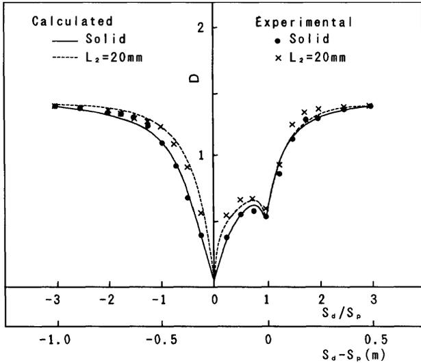
Figure 3. Relationship between brush speed and image density. Experimental conditions (Developer A:  $S_p$ , 254 mm/s;  $V_b$ , 400 V;  $V_p$ , 50 V;  $G_{doc}/G_{dev}$ , 0.8/1 mm;  $\Phi_b$ , 57 mm), calculated conditions ( $P_1 \cdot u/\psi$ , 0.22;  $\lambda$ , 2.1;  $v$ , 0.71;  $M_0$ , 1 mg/cm<sup>2</sup>;  $D_p$ , 0.08;  $D_s$ , 1.46;  $M_s$ , 0;  $M_r$ , 0.06 mg/cm<sup>2</sup>;  $\mu$ , 0.35;  $W$ , 4 mm;  $L_1$ , 60 mm;  $L_2$ , 20 mm).
