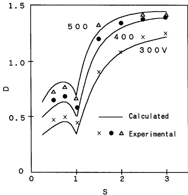
Figure 5. Influence of development bias voltages. Experimental and calculated conditions ( $V_p$ , 75 V;  $M_0$ , 0.64, 0.93, and 1.22 mg/cm<sup>2</sup> for  $V_b = 300, 400,$  and 500 V; other conditions are as in Fig. 3).
