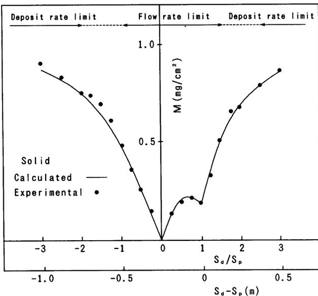
Figure 4. Relationship between brush speed and developed toner mass for solid images. Experimental and calculated conditions are as in Fig. 3.
