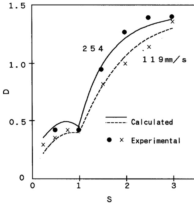
Figure 7. Influence of process speeds. Experimental conditions (Developer B;  $V_b$ , 400 V;  $V_r$ , 50 V;  $G_{doc}/G_{dev}$ , 1.3/1.6 mm;  $\Phi_b$ , 40 and 57 mm for  $S_p = 119$  and 254 mm/s); calculated conditions ( $P_1 \cdot u/\psi$ , 0.15 and 0.17 for  $S_p = 119$  and 254 mm/s;  $\lambda$ , 1.8;  $v$ , 1.78 and 0.83 for  $S_p = 119$  and 254 mm/s;  $M_0$ , 1 mg/cm<sup>2</sup>;  $W$ , 3.1 and 3.5 mm for  $S_p = 119$  and 254 mm/s; other conditions are as in Fig. 3).
