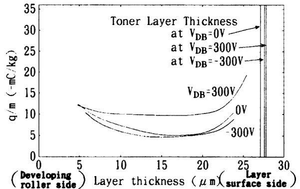
Figure 9. Charge distributions in the toner layer in thickness direction at  $V_{DF} = 200V$ .
