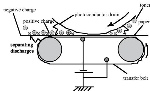
Figure 1. The schematic diagram of the belt transfer system.
