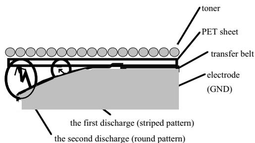
Figure 9. Mechanism of the second discharge.
