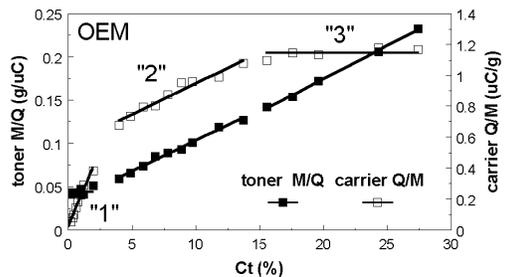
Figure 4. OEM toner mass-to-charge ( $M/Q$ ) and carrier charge-to-mass ( $Q/M$ ) ratios as a function of toner concentration,  $C_t$ .
