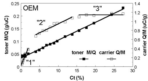
Figure 3. OEM toner mass-to-charge ( $M/Q$ ) and carrier charge-to-mass ( $Q/M$ ) ratios as a function of toner concentration,  $C_t$ .
