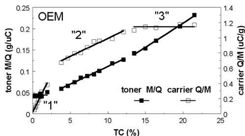
Figure 6. OEM toner mass-to-charge ( $M/Q$ ) and carrier charge-to-mass ( $Q/M$ ) ratios as a function of toner concentration,  $TC$ .
