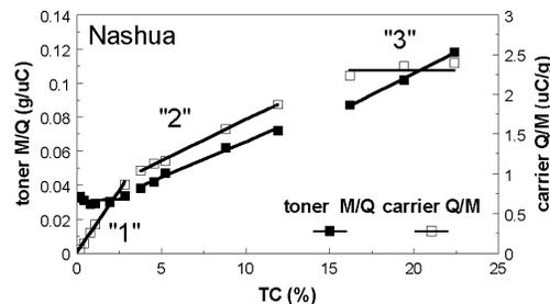
Figure 7. OEM toner mass-to-charge ( $M/Q$ ) and carrier charge-to-mass ( $Q/M$ ) ratios as a function of toner concentration,  $TC$ .
