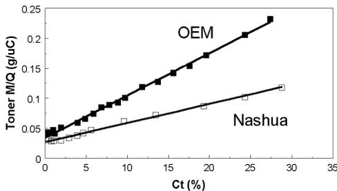
Figure 2. OEM and Nashua mass-to-charge ratios,  $M/Q$ , as a function of toner concentration,  $C_t$ .
