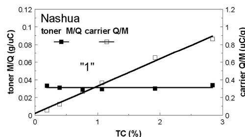
Figure 8. OEM toner mass-to-charge ( $M/Q$ ) and carrier charge-to-mass ( $Q/M$ ) ratios as a function of toner concentration,  $TC$ , in region “1”.
