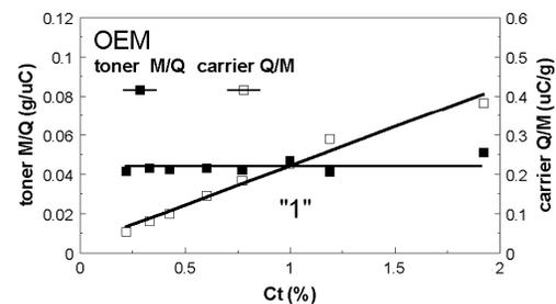
Figure 5. OEM toner mass-to-charge ( $M/Q$ ) and carrier charge-to-mass ( $Q/M$ ) ratios as a function of toner concentration,  $C_t$ , in region "1".
