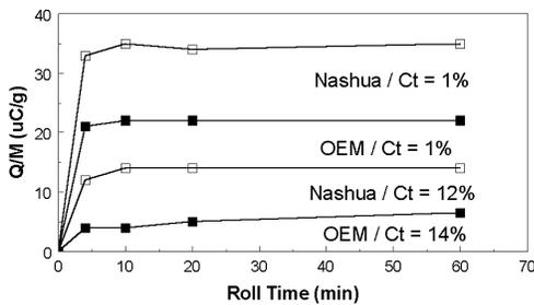
Figure 1. OEM and Nashua toner charge-to-mass ratios,  $Q/M$ , as a function of roll time at two different toner concentrations,  $C_t$ .
