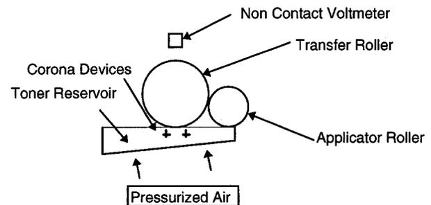
Figure 1. Block Diagram of Q/M Measurement Configuration.
