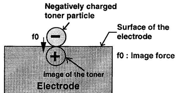
Figure 2. A charged toner particle adhered on the surface of the electrode.
