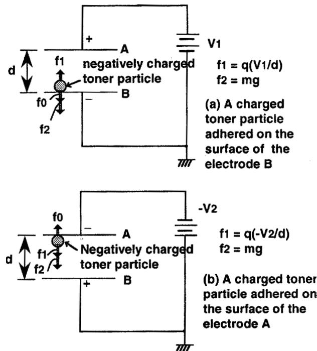
Figure 3. Detailed schematic expression of the parallel electrodes.
