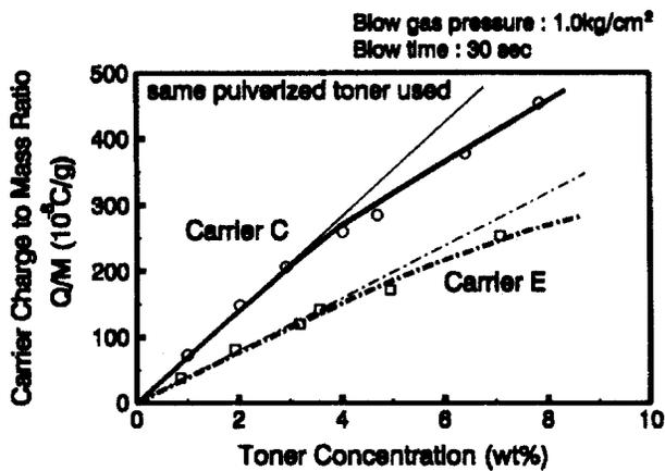
Figure 1. Relationship between carrier charge-to-mass ratio and toner concentration.
