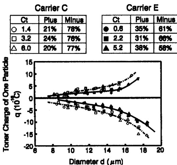
Figure 3. Measurements of the toner charge as a function of particle diameter for three toner concentration.
