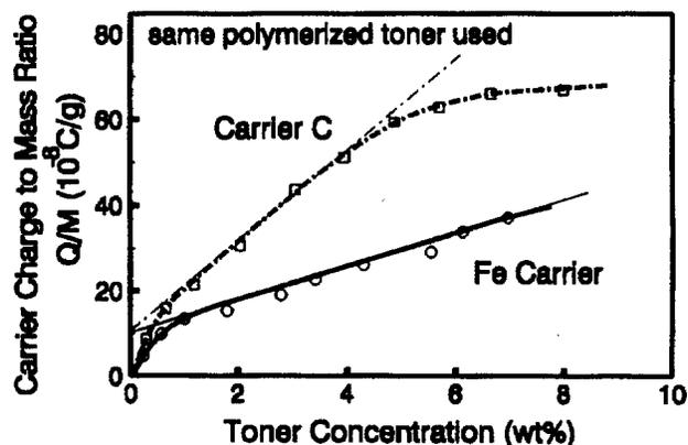
Figure 4. Relationship between carrier charge-to-mass ratio and toner concentration.
