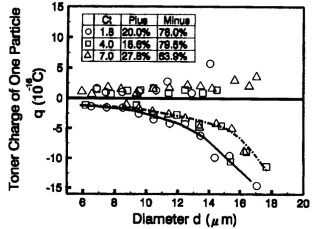
Figure 6. Measurements of the toner charge as a function of particle diameter for three toner concentration.
