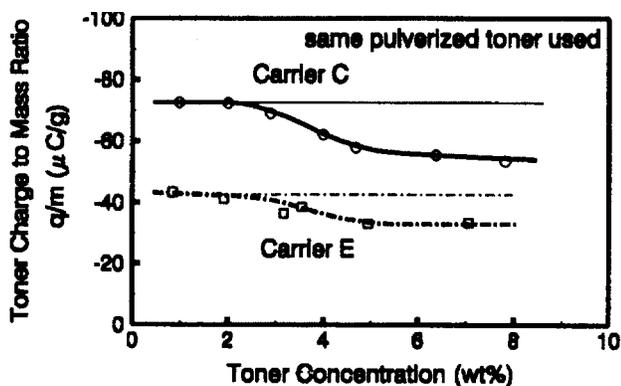
Figure 2. Relationship between toner charge-to-mass ratio and toner concentration.
