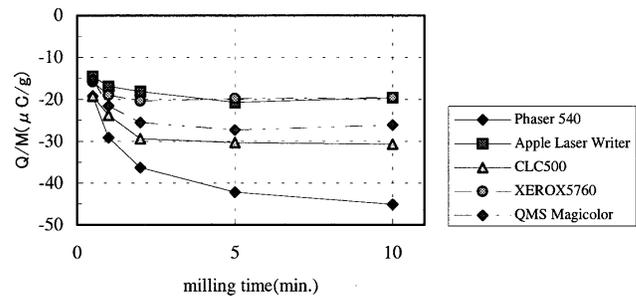
Figure 7. The charge-up behavior of the various color toners. Carrier: Silicone coated ferrite (T/D = 3%).
