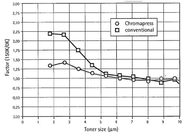
Figure 3. Particle enrichment in 150K-old developer mix.
