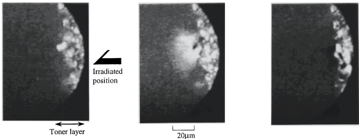
Figure 2. Pictures of irradiated part of toner layer
