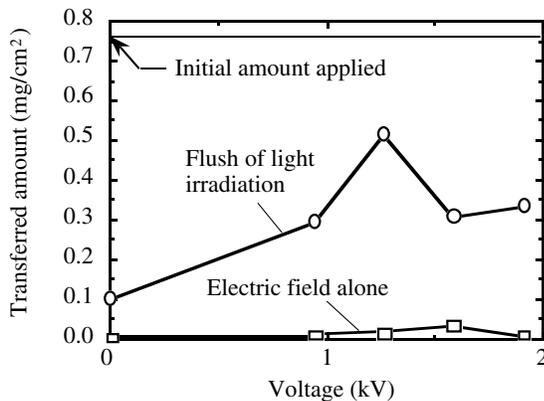
Figure 4. The amount of transferred toner as a function of the voltage supplied to parallel electrodes.
