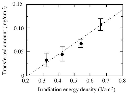
Figure 3. The amount of transferred toner as a function of the irradiation energy density.
