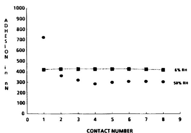
Figure 9. RH response of adhesion of toner with 100% surface coverage of 30 nm hydrophobic titania.
