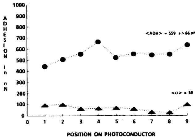
Figure 2. Adhesion of toner with 100% surface coverage of low BET ( $50 \text{ m}^2/\text{g}$ ) hydrophobic silica at  $70^\circ$ , 50% RH. Average adhesion values in solid circles. Standard deviations in solid triangles.
