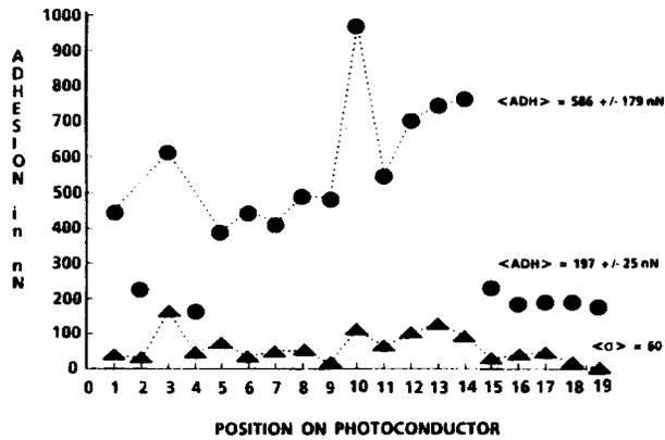
Figure 1. Adhesion of toner with 50% surface coverage of low BET ( $50 \text{ m}^2/\text{g}$ ) hydrophobic silica at  $70^\circ$ , 50% RH. Average adhesion values in solid circles. Standard deviations in solid triangles.
