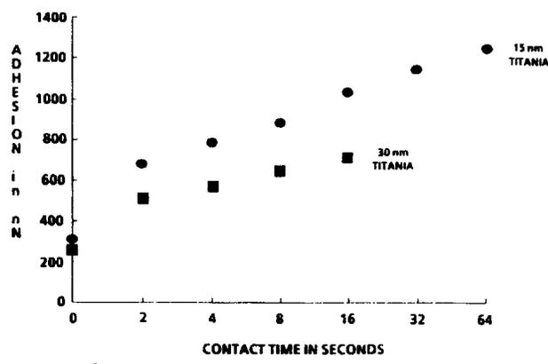
Figure 8. Adhesion increase as function of contact time at 70°, 50% RH for toners coated with 100% surface coverage of 15 nm and 30 nm hydrophobic titanias.
