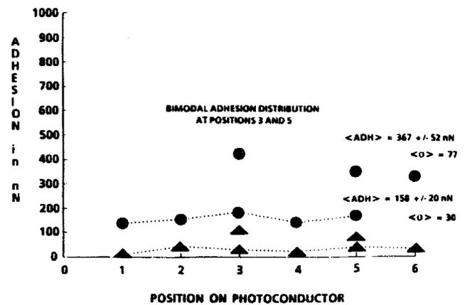
Figure 6. Adhesion of toner with 100% surface coverage of high BET ( $200 \text{ m}^2/\text{g}$ ) hydrophobic silica at  $70^\circ$ , 20% RH. Average adhesion values in solid circles. Standard deviations in solid triangles.
