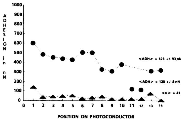
Figure 3. Adhesion of toner with 100% surface coverage of hydrophilic silica at  $70^\circ$ , 50% RH. Average adhesion values in solid circles. Standard deviations in solid triangles.
