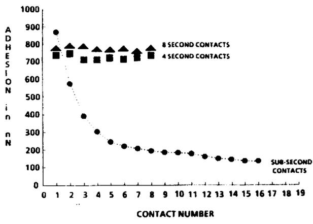
Figure 7. Adhesion of toner with 100% surface coverage of high BET 15 nm titania at 70°, 50% RH.
