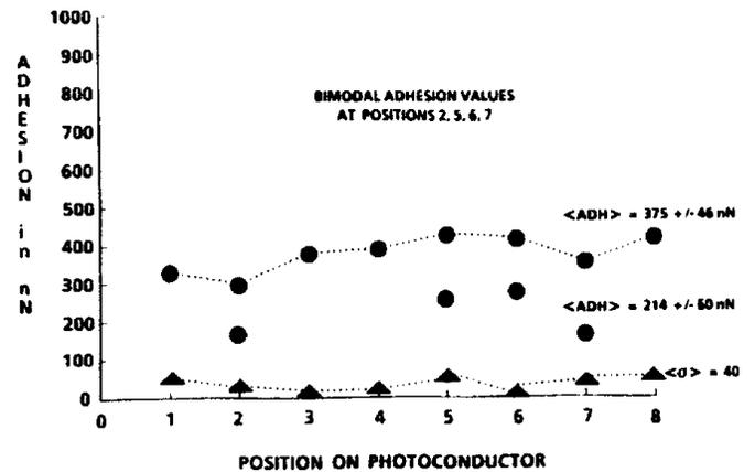
Figure 5. Adhesion of toner with 50% surface coverage of high BET ( $200 \text{ m}^2/\text{g}$ ) hydrophobic silica at  $70^\circ$ , 20% RH. Average adhesion values in solid circles. Standard deviations in solid triangles.
