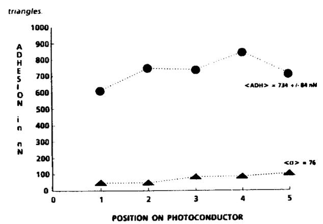
Figure 10. Adhesion of toner with 100% surface coverage of hydrophilic titania at 70°, 50% RH. Average adhesion values in solid circles. Standard deviations in solid triangles.
