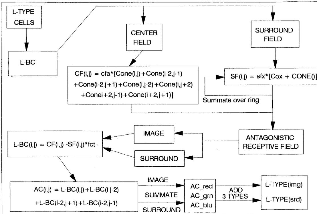
Figure 6. Compute L-Type Cell Response
