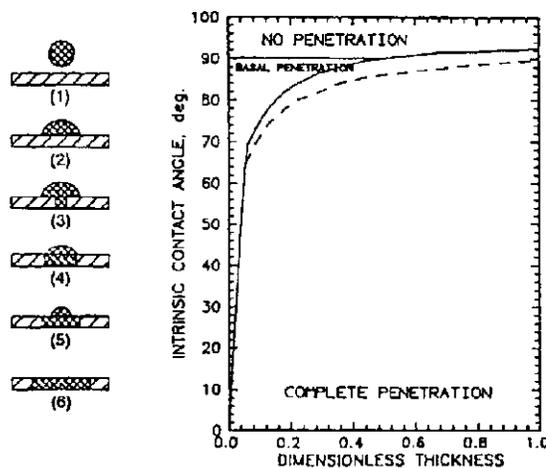
Figure 2. Theoretically calculated drop penetration modes for a thin porous medium simulating paper (Ref. 5)
