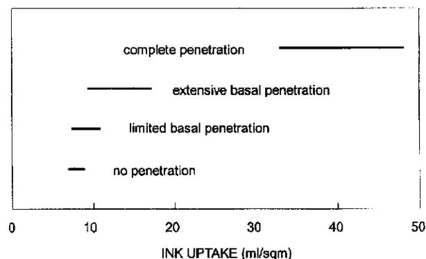
Figure 3. Liquid volume uptake for papers of different penetration characteristics
