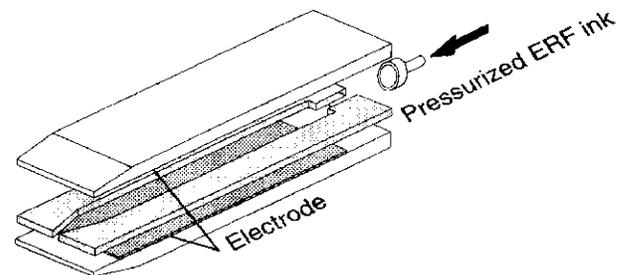
Figure 1. Schematic diagram of the print head
