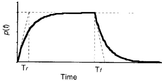
Figure 4. Effective pressure exerted to ER fluid
