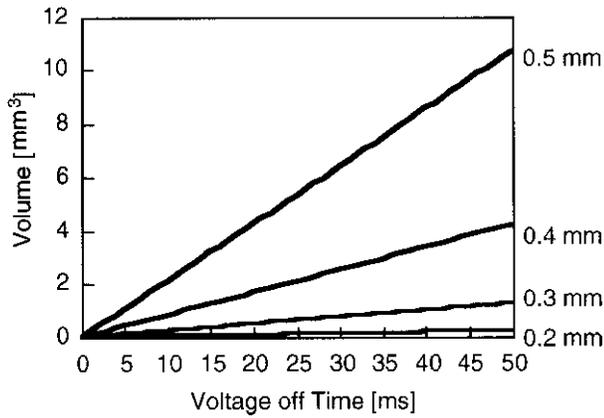
Figure 6. Ejected droplet volume vs. electric field off time with different nozzle aperture
