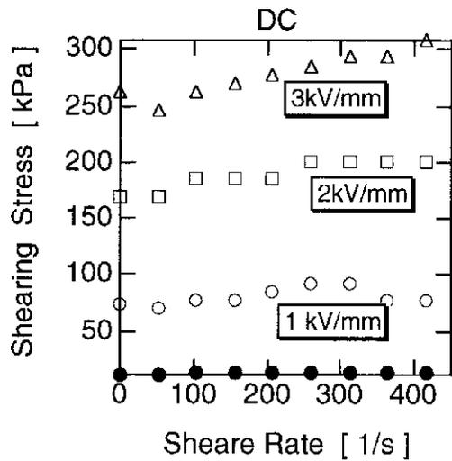
Figure 2. Shearing stress vs. shear rate for ERF with different static electrical field
