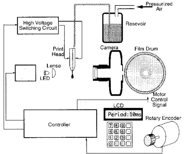
Figure 5. Experimental setup for measuring droplet volumes
