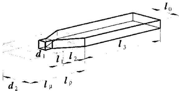
Figure 3. Shape of ink channel and variables
