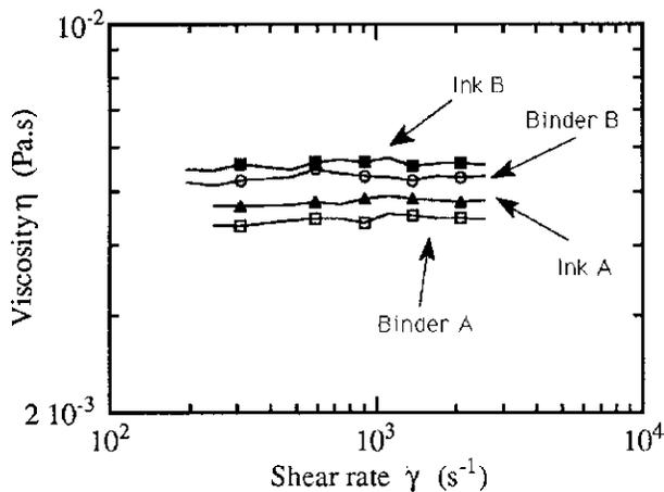
Figure 1. Shear viscosities of binders and inks
