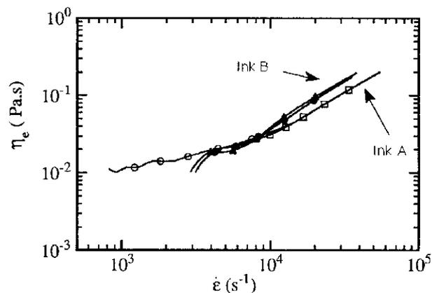
Figure 4. Variation of apparent elongational viscosity as a function of strain rate
