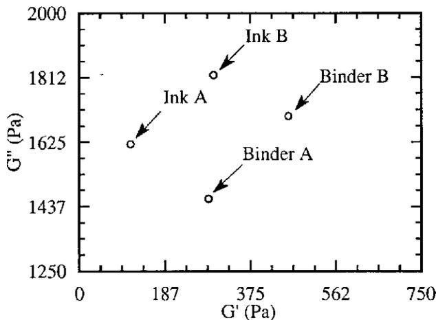
Figure 2. Cole-Cole diagram of the viscoelastic moduli of the binders and inks
