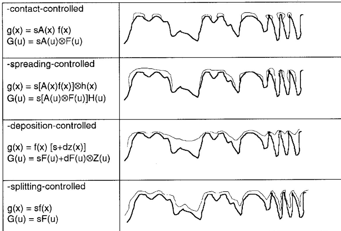
Figure 2. Mechanisms of ink transfer.
