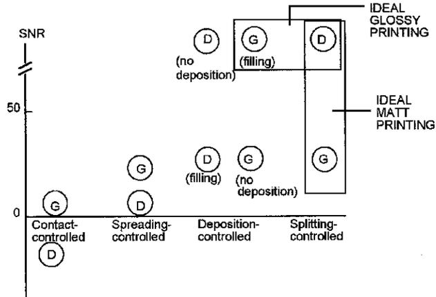
Figure 3. SNR of density (D) and gloss (G) when ink transfer is controlled by different mechanisms.
