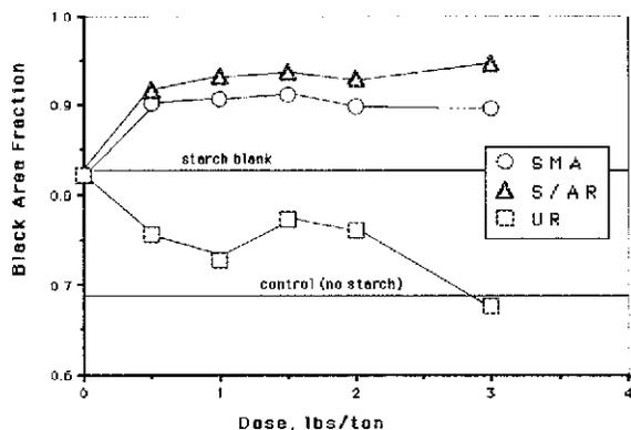
Figure 6. Dependence of Toner Adhesion on Surface Treatment.
