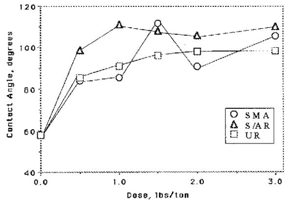
Figure 4. Dependence of Initial Contact Angle on Surface Treatment.
