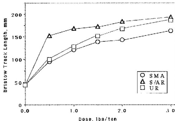
Figure 3. Dependence of Bristow Track Length on Surface Treatment.
