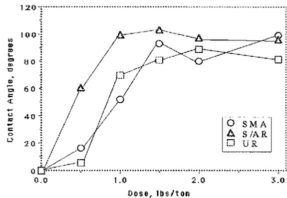
Figure 5. Dependence of Contact Angle at 60° on Surface Treatment.
