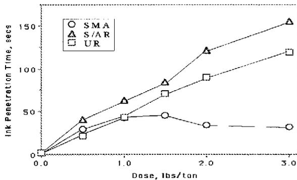
Figure 2. Dependence of Ink Penetration Time on Surface Treatment.
